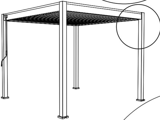
Place the reference card to the right position as shown. Drill a 14mm hole at the marked position.
