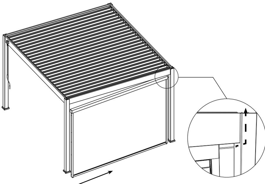
**Insert the cable through the hole, take the cable and pull out tightly to avoid any entanglement.**
