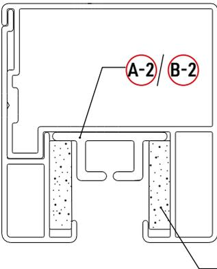
When installing the electric screen, you must ensure that the foam is inserted into the groove of the A-2/B-2.
