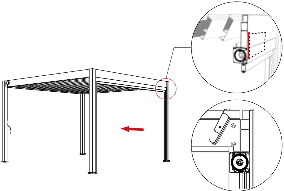
Put the frame up and make sure the outer face of wind screen box aligns with the outer face of the beam.
