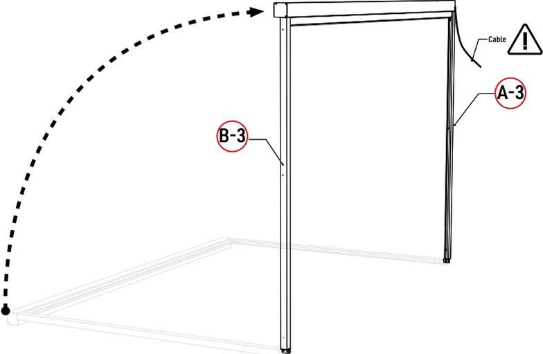
**Place the screen frame to the pergola. Make sure that the cable side aligns with the hole.**
