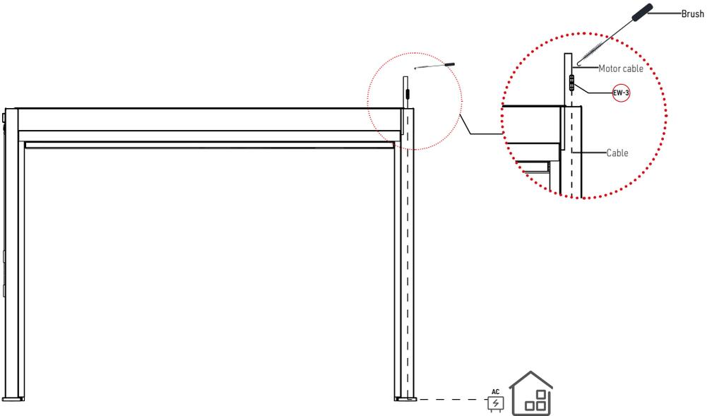
1. Insert the two cables into the post after connection;
